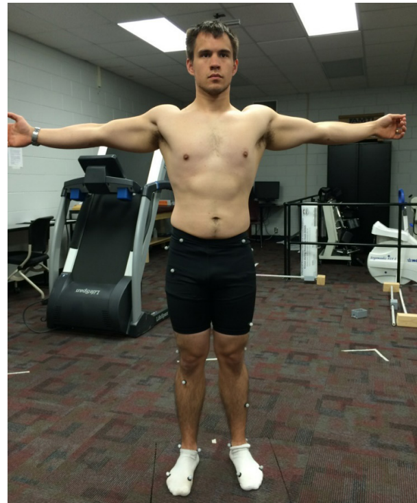
Figure 1a. Anterior view of retroreflective markers placed at the 1 st metatarsal head, 5 th metatarsal head, calcaneal tuberosity, lateral malleolus, medial malleolus, mid-tibia (shank), lateral knee joint line, mid-femur (thigh), greater trochanter of the femur, anterior superior iliac spine, posterior superior iliac spine and sacrum
